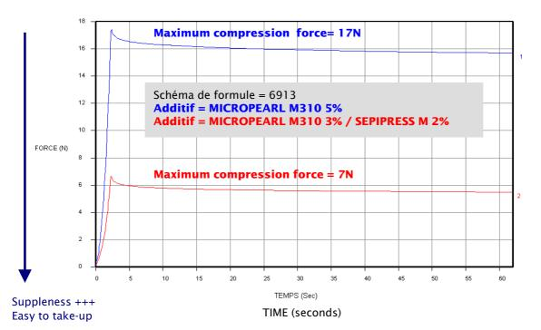
Maximum compression force: force necessary to penetrate inside the product with a fixed speed and depth. Higher is the force, harder is the pressed powder.
